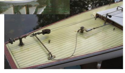
Stern deck detail note; spring tensioned pulley, the rudder arm is operated by a brass rod from an internal servo.
