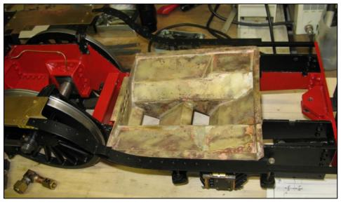
This arrangement precludes the fitting of any "normal" dropping ash pan and grate.
