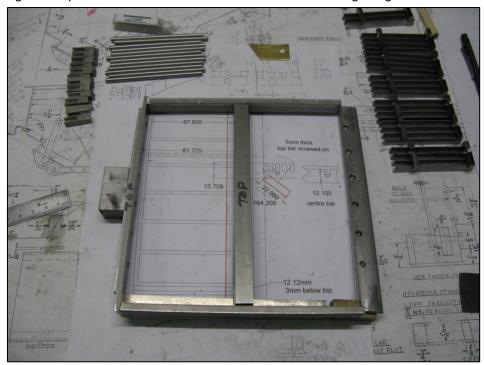
As no design for a model version existed as far as I could tell I set to and designed my own. It consists of a stainless-steel frame with a centre bar giving two sides into which fit six individual grate units.
